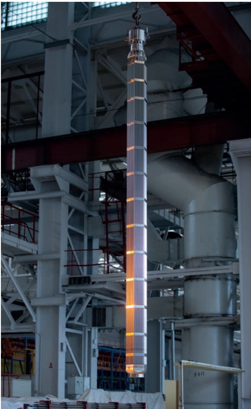
Figure 5A-1. A fuel assembly of the AES-2006 nuclear power plant.
