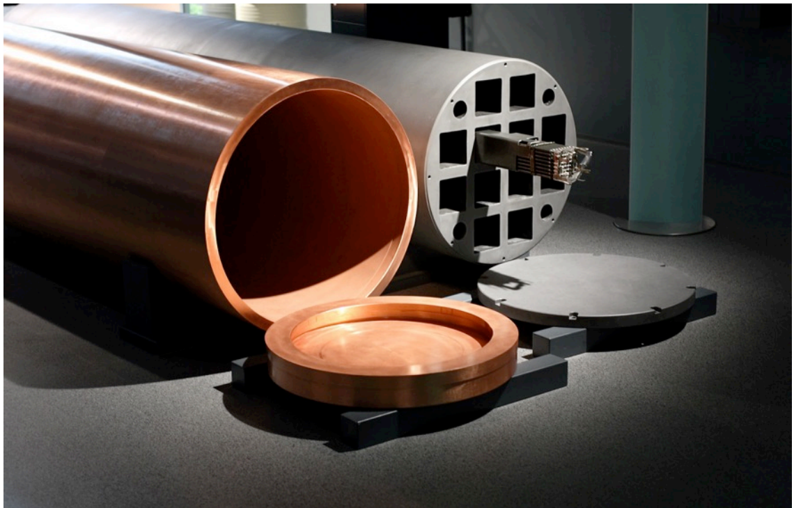
Figure 3-6. The insert and outer shell of a disposal canister. The image shows a canister for the spent nuclear fuel from the Olkiluoto 1 and 2 reactors. It has a diameter of 1.05 meters and is 4.8 meters long. Figure by Posiva Oy. The Fennovoima canisters will be slightly longer and have a different type of insert.
