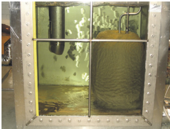
Figure 5.5. A full-scale filter element in LUT's containment sump experiment. The insulation wool in the circuit had accumulated in the filter element during the experiment. (Photo: Jani Laine).
