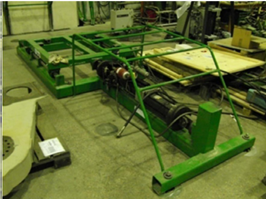
Figure 5.8. VTT's hydraulic vibration table for earthquake testing.
