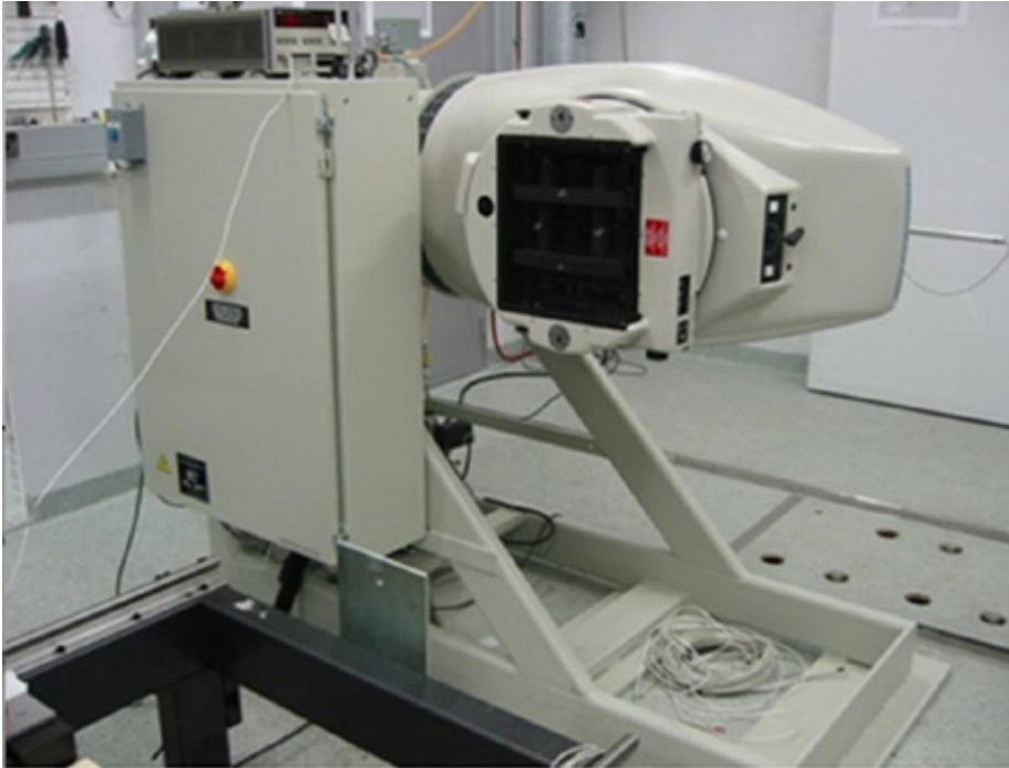
Figure 5.16. ^{60}\text{Co} gamma irradiator GBX200 with 400 TBq radiation source activity.
