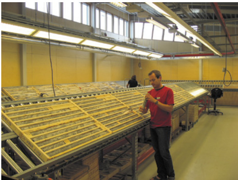
Figure 5.13. Posiva Oy's site investigation. Core drilled samples taken of the Olkiluoto bedrock, and other core samples collected for final disposal site investigation, are mapped and processed in the research hall located at the Olkiluoto research site. In the picture, processing of core drilled samples in 2007. (c) Posiva Oy. Photo: Sari Ojala.
