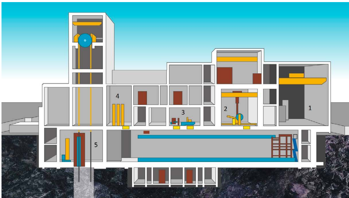
■ Figure 4. Longitudinal cross-section of the encapsulation plant. On the right, there is the reception and storage room for transport containers and transfer casks (1). To the left, there are the fuel handling cell (2), copper lid welding machine and the machining and inspection station (3), reception and storage facility for empty canisters (4) and the canister lift (5).
