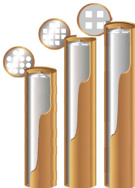
■ Figure 4. Final disposal canisters for the different fuel types: pictured are the canister types for Loviisa 1–2 (VVER 440) on the left, Olkiluoto 1–2 (BWR) in the middle and Olkiluoto 3 (EPR, OL3) on the right.
