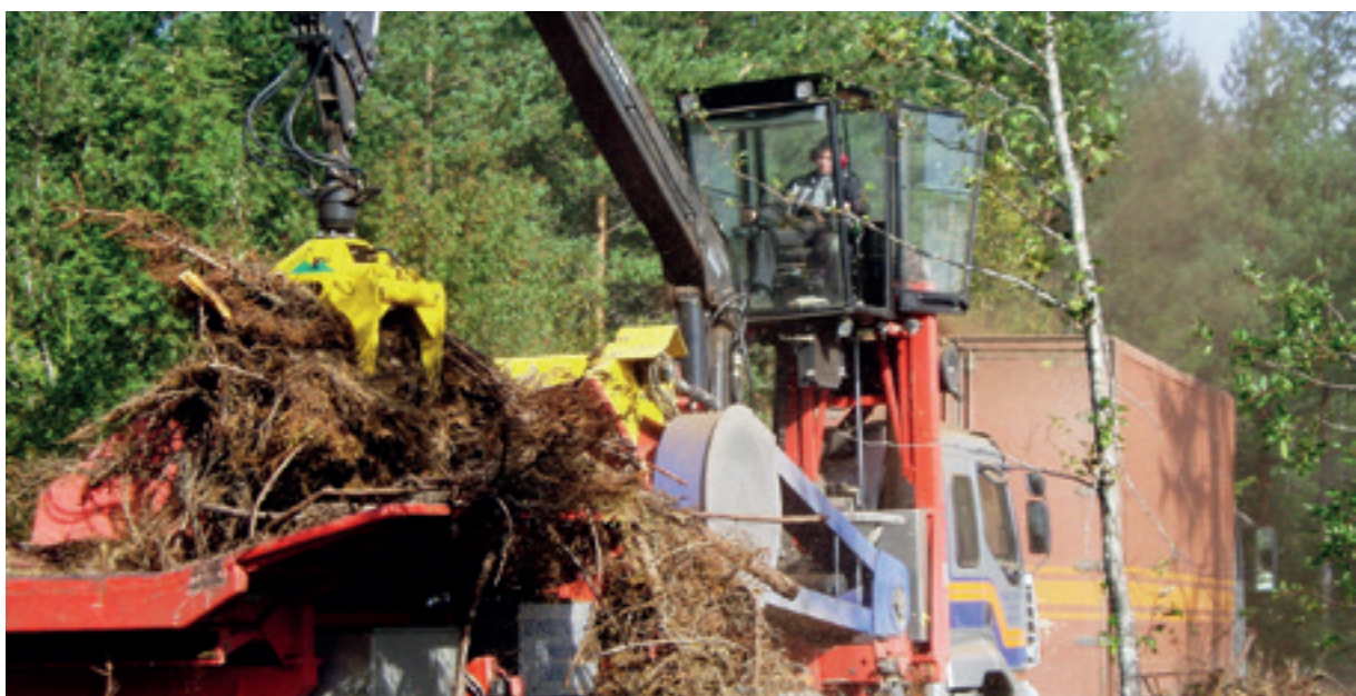
Chipping of logging residues (LHM Hakkurit Oy)
