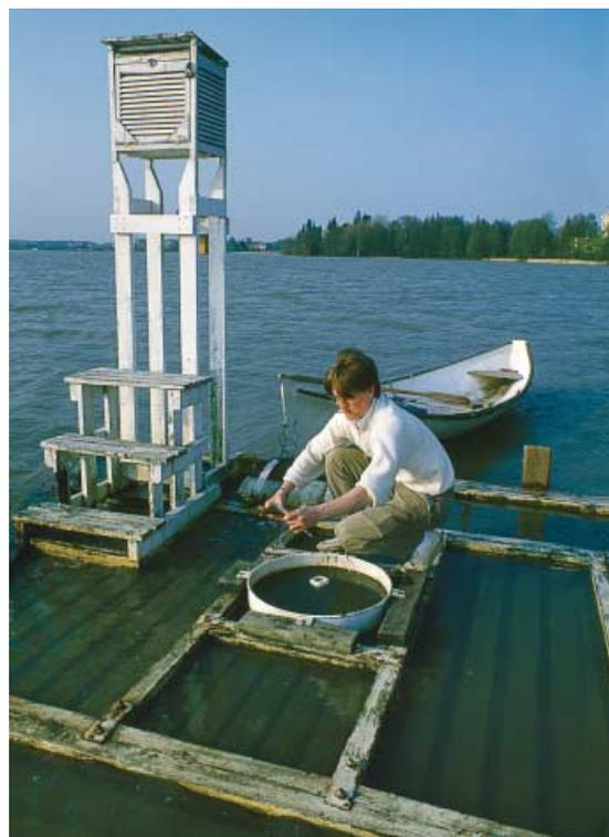
**Up to 50 cm of water can evaporate** from Finland's lakes during the summer. This has been ascertained using triangular rafts, in use for instance on Lake Tuusula.
