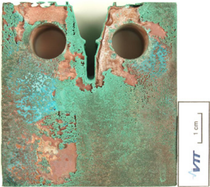
Figure 7. Extensive general corrosion in the CT specimen after 4400 h (90°C) in aerated simulated Olkiluoto groundwater.
