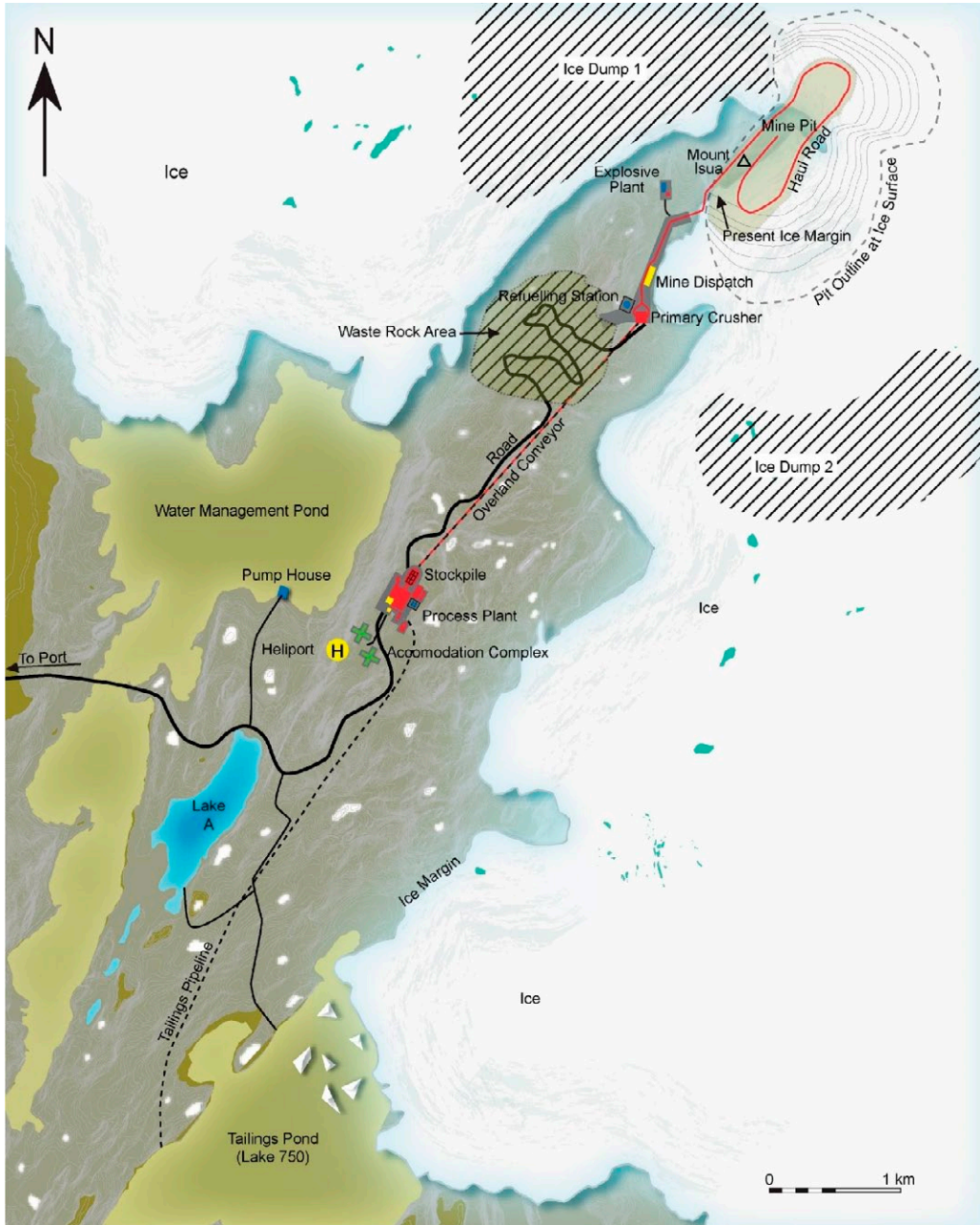
Figure 23. Map of a possible production of iron ore from Isua. The open mine will be surrounded by ice on three sides. Lake 750 is planned for tailings. After Orbicon A/S (2013).
