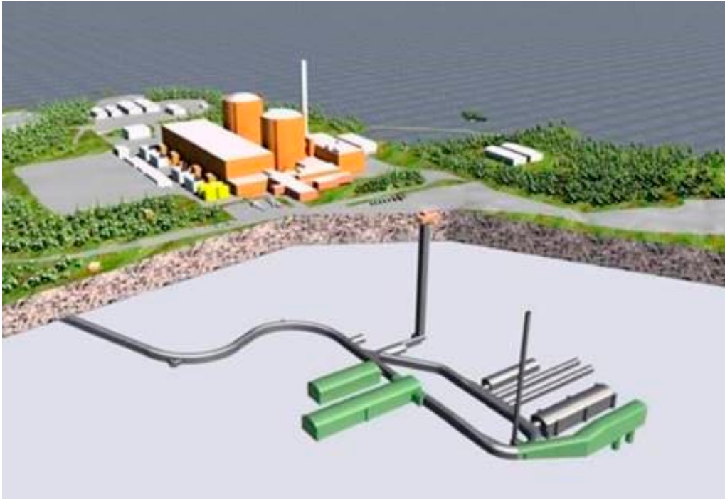
Figure 5. LILW disposal facility in Loviisa. The rooms in use are marked in dark grey and the planned extension is marked in green. (Source: Fortum).
